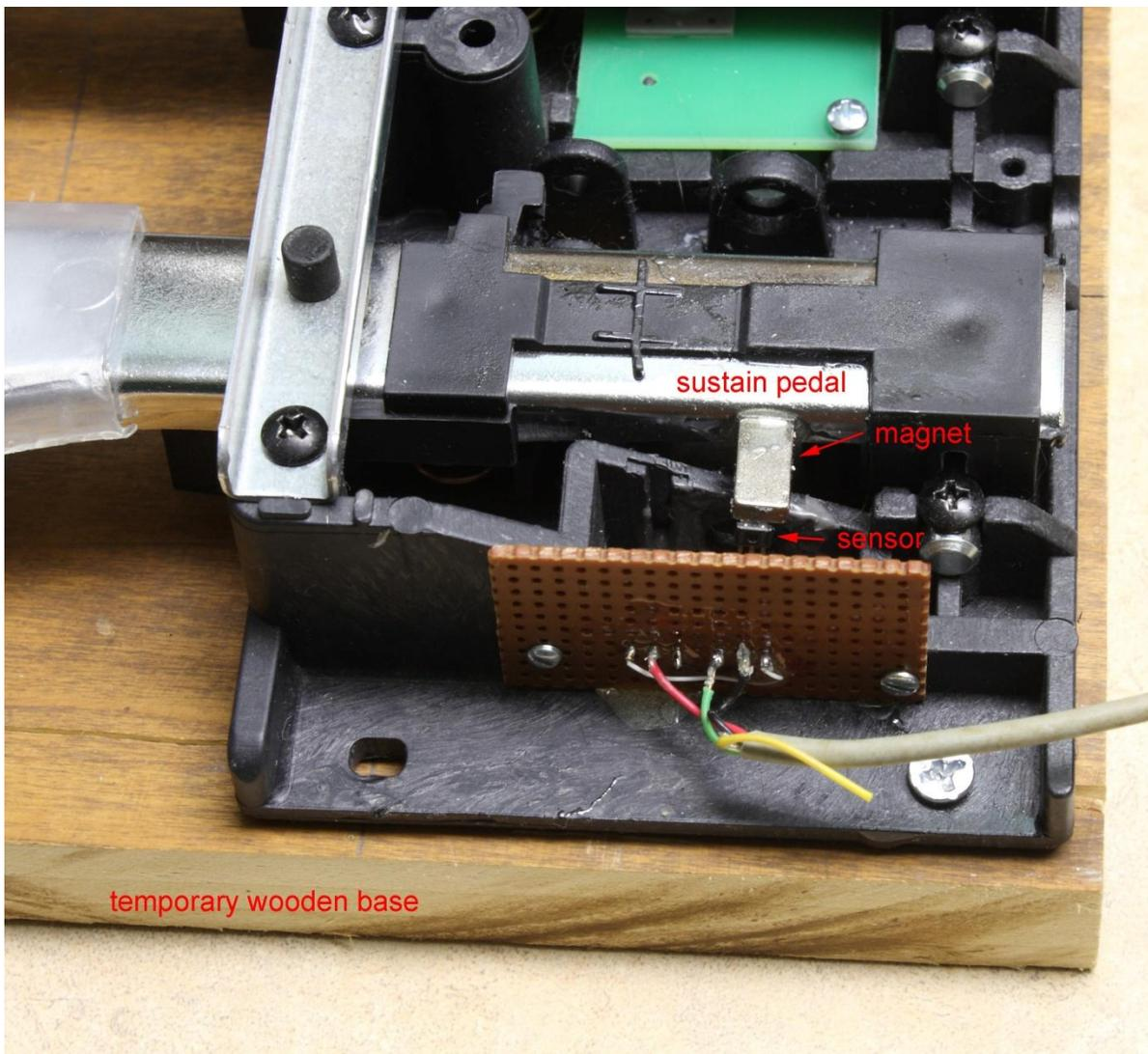
Perfboard in place on pedal, replacing pot.
